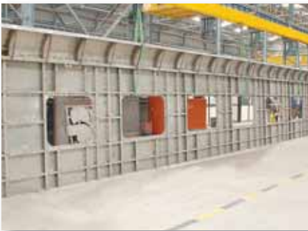
LHB - Side Wall (Inner view)
